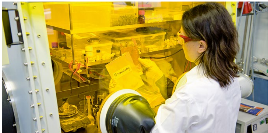
Figure 1 Production of test cells with new battery materials (© K. Dobberke, Fraunhofer ISC)
