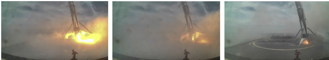
Fig. 3 The accident caused by the position and other state errors of the rocket
