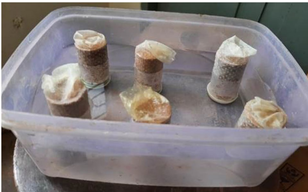
Fig. 9 UCS samples kept for soaking for 24 hours
