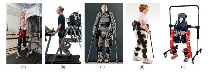
Fig. 10 Representative of medical rehabilitation LEEX: a LOPES II [130] b ALEX III [131] c Ekso-GT [132] d Indego [133] e Atlas 2030 [134]
