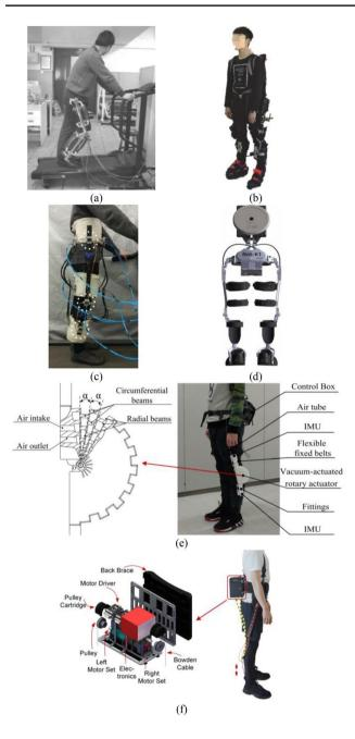
**Fig. 7** Representative CLEEX in China: **a** Pneumatic muscles exoskeleton, Harbin Engineering University [111] **b** rope driven exoskeleton, the SIAT of the CAS [112] **c** flexible exoskeleton, Southeast University [114] **d** Ant-K1, Kenqing Technology [115] **e** soft knee exoskeleton, Beijing Institute of Technology [116] **f** exosuit, SIACAS [117]
