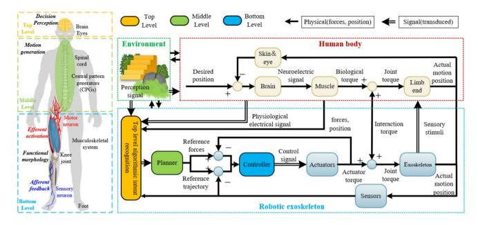
Fig. 16 Control diagram of the human-exoskeleton environment-coupled system
