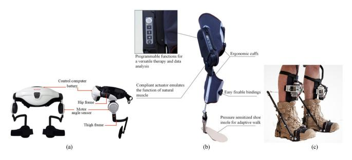
Fig. 2 Single joint lower extremity exoskeleton systems. a Walking Assist [58] b MAK [60] c Autonomous leg [62]
