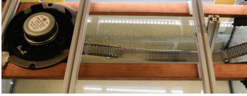
Fig. 3 Experimental set-up showing the water basin, the loudspeaker and the horizontally arranged metallic tape.
