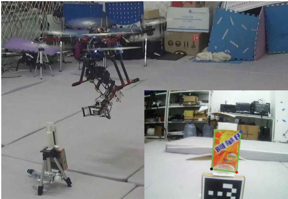
Fig. 1 Aerial manipulator system with a 6-DoF serial manipulator equipped under a co-axis octocopter. The bottom-right sub-figure shows an image of the target from the camera’s view.
