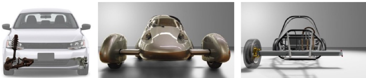
Fig. 4 Alternate construction details of the VLC, in particular showing how elimination of the shock tower can enable improved aerodynamics
