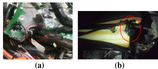
Fig. 17 Results of testing of the contact area between motor controller and seat. a Damaged area of motor controller. b Hinged plate of seat
