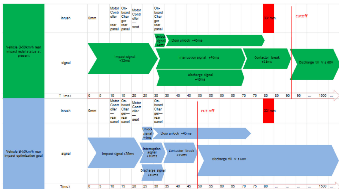
Fig. 23 Control signal transmission times
