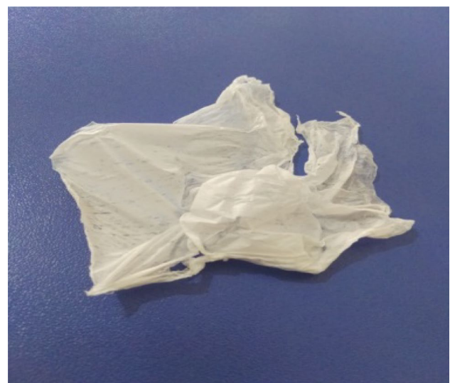
Fig. 6 Macroscopic image of kefiran/PVA nanofibers
