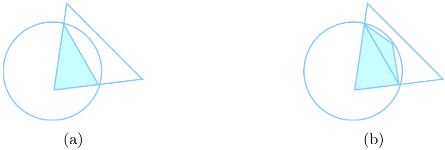
Fig. 2 If a finite element triangle is only partially covered by an Euclidean ball, the intersection contains circular caps. The nocaps ball (a) omits this cap, whereas the approxcaps ball (b) retriangulates the whole intersection
