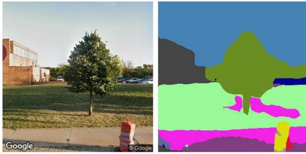
Fig. 3 Example of GSV and Semantic segmented images: (left) GSV image and its corresponding (right) semantic segmented image. In the semantic segmented image light-blue color represents as sky, green color as trees, light green color as grass, gray color as pole, dark-gray as building, pink color as sidewalk, blue color as cars, and purple color as road respectively
