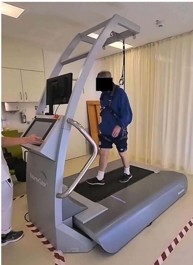
Fig. 1 Patient walking on the perturbation treadmill secured by a safety harness
