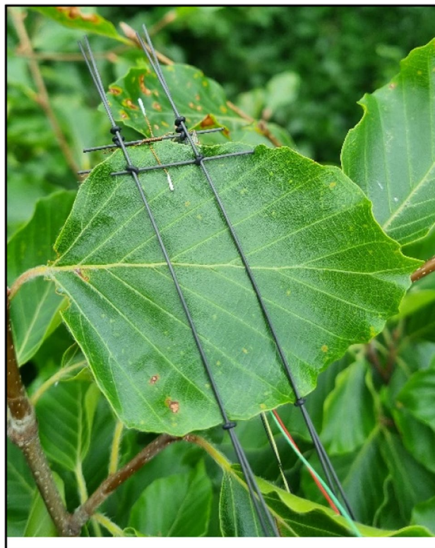
Fig. 2 The LAT-B2 [47] leaf temperature sensor which was positioned in the upper tree crown and used to validate the TIR imagery
