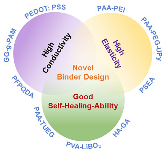
Fig. 19 Schematic of multiple binders for Si-based electrodes
