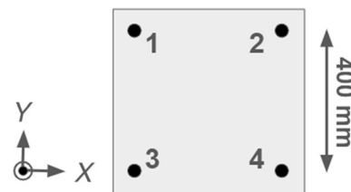
Fig. 4 Coordinate system and actuator layout for each panel. Once tip, tilt, and piston values are extracted, they must be converted to actual numbers of rotations on the actuators
