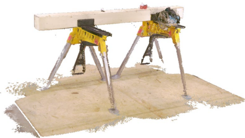
Fig. 22 Raw point cloud of the scanned preprocessed timber piece to compare with the mesh reconstructed by TSLAM. The object was scanned twice on both sides and then aligned and combined
