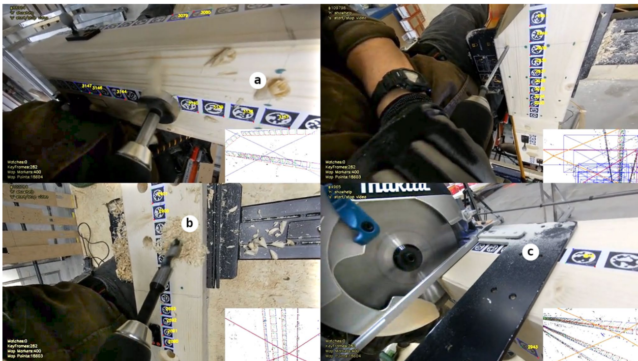
Fig. 10 Views of fabrication sequences during tracking by TSLAM. Due to the tags' redundancy, TSLAM is capable of performing self-localization against a chips and generated blur; b accumulation of
