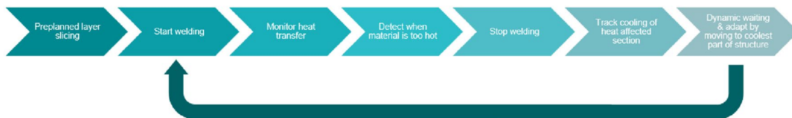
Fig. 12 Process diagram for ECS informed adaptive path planning
