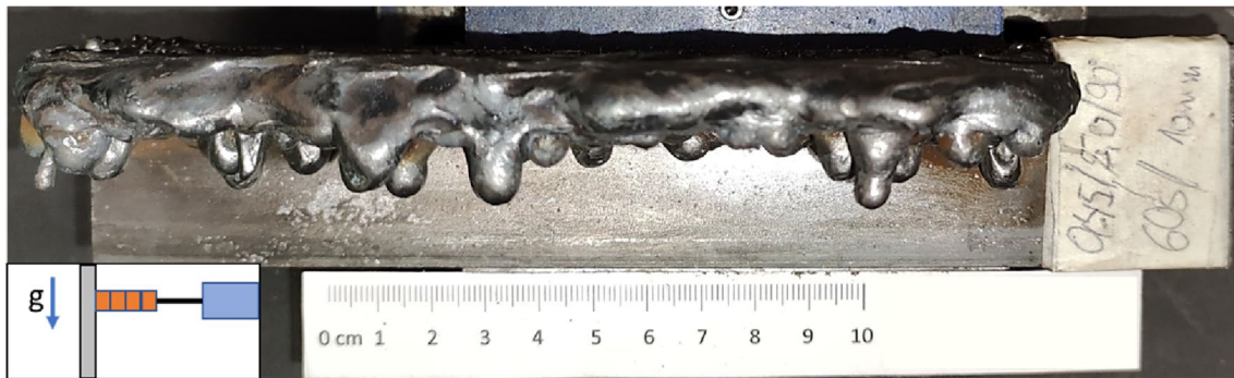
Fig. 7 Exemplary weldment at a 90° angle
