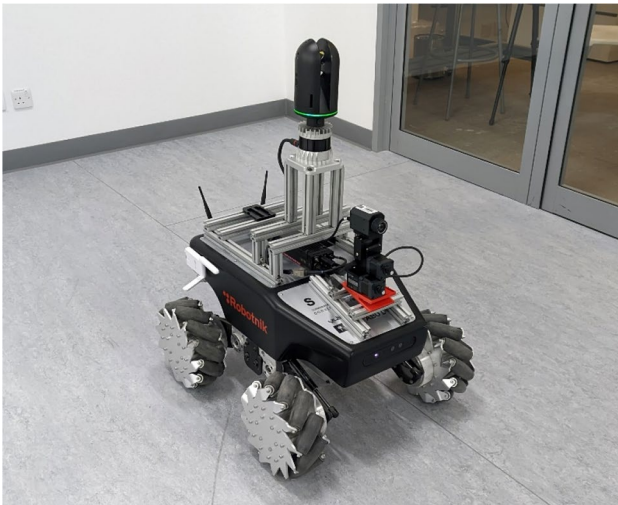
Fig. 15 SUMMIT-XL ARS platform with customized payload
