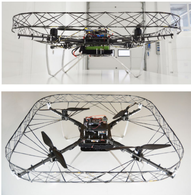
Fig. 4 The UAV was the result of four successive prototypes and gradually tailored towards stable flight, low self-weight, a payload of at least 2 kg, and scalable self-localization
