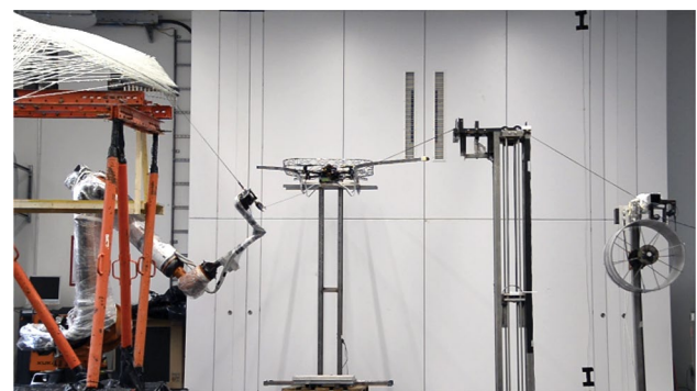
Fig. 7 The tension mechanism is high tension mode: the dancer provides high consistent tension on the fiber line, and the rotation of the drum can lift the dancer further if necessary
