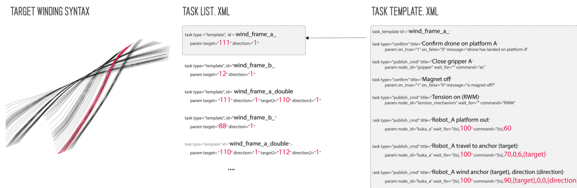
Fig. 12 A given fiber syntax in the CAD environment is compiled into a task list of sequential XML instructions. Any reoccurring sequence could be grouped together as a “template”. To recompile the task list, a different set of task templates would need to be uti-
