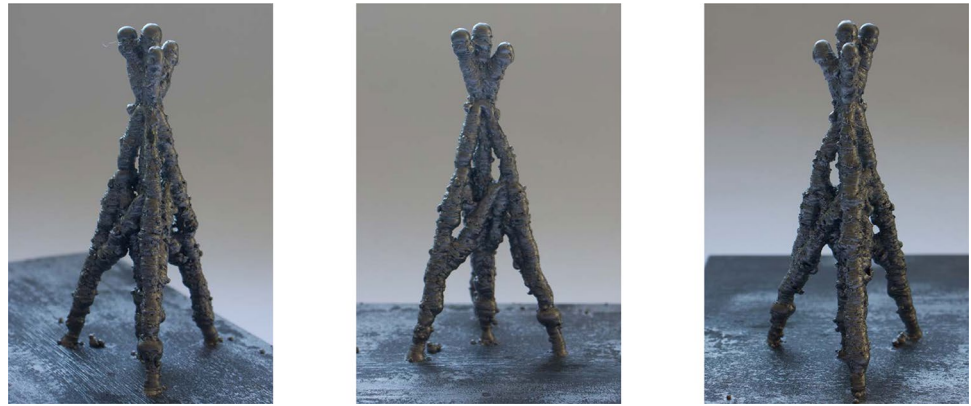
Fig. 9 Result of complex branching experiment testing different branching and joining cases from different points of view
