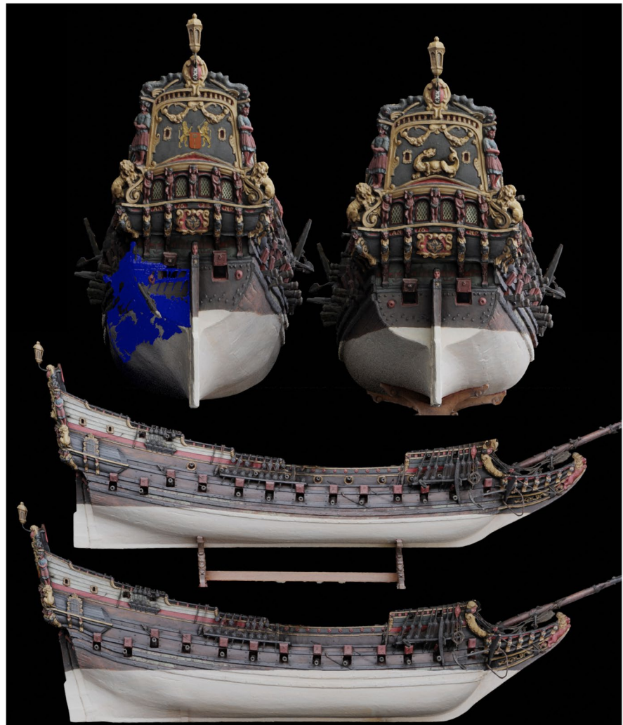
Fig. 13 Reconstructing Batavia III by modifying the N16 scan. Sterns are shown above with Batavia III (top left, including scan data) and N16 (top right) and an orthographic starboard view of N16 (middle) and Batavia III, with deeper hull and fewer gun ports (bottom). (Image by John McCarthy, 2020.)
