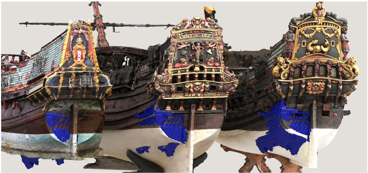
Fig. 10 Comparison of the scans of the archaeological remains of Batavia (in blue) with the full-size Batavia II reconstruction and the scaled-up models of Prins Willim and the N16 model. (Image by John McCarthy, 2022.)
