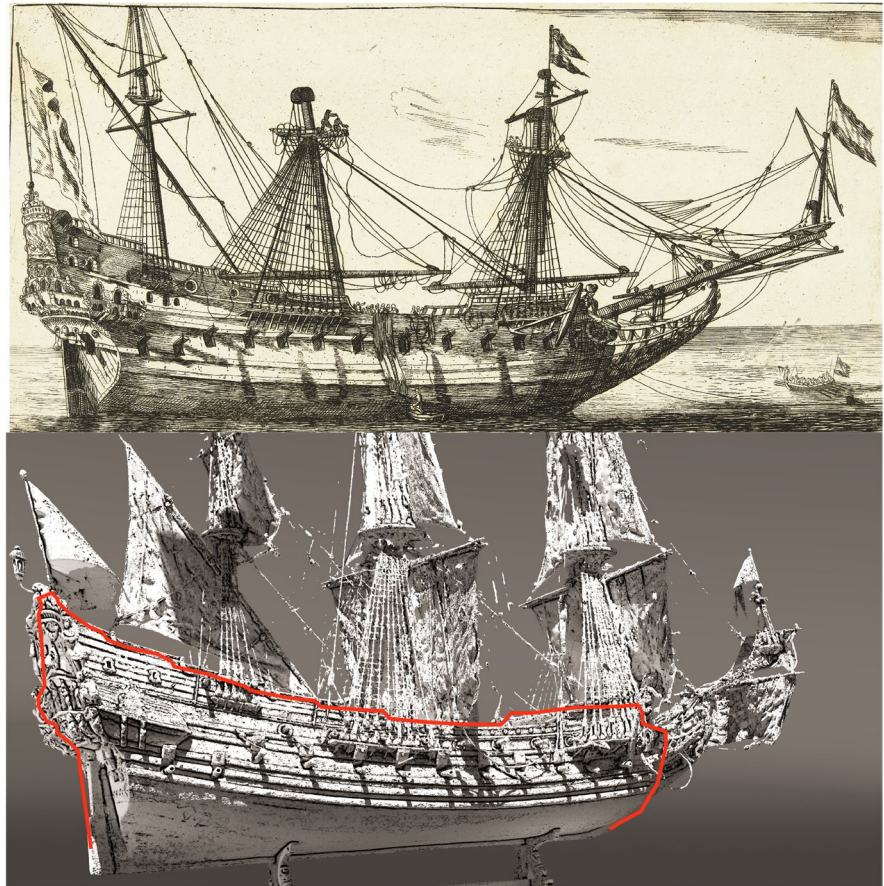
Fig. 4 Comparison of Reinier Nooms’s etching of the VOC ship Salamander (above) (Nooms 1652–1654) with an untextured “ambient occlusion” rendering of the 3-D scan of the N16 model (below) from the same angle. (Image by John McCarthy, 2022.)
