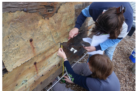
Fig. 6 Lauren Davison and Peta Fray recording hull remains at QEP using baseline-offset measurements. (Photo by Mark Polzer, 2014.)
