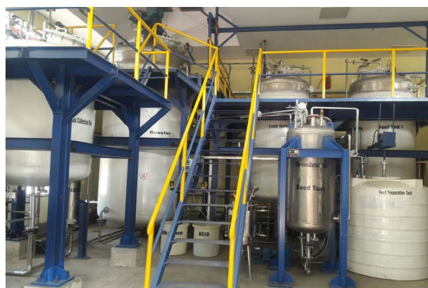
Fig. 4 10,000 L pilot plant for biohydrogen production at Department of Biotechnology, IIT Kharagpur
