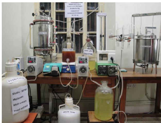
Fig. 3 20 L Prototype mole for demonstration of continuous biohydrogen production at Department of Biotechnology, IIT Kharagpur
