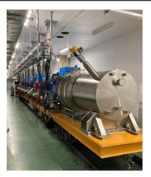
Fig. 11 (Color online) The first SHINE 1.3 GHz cryomodule prototype in the horizontal test tunnel
