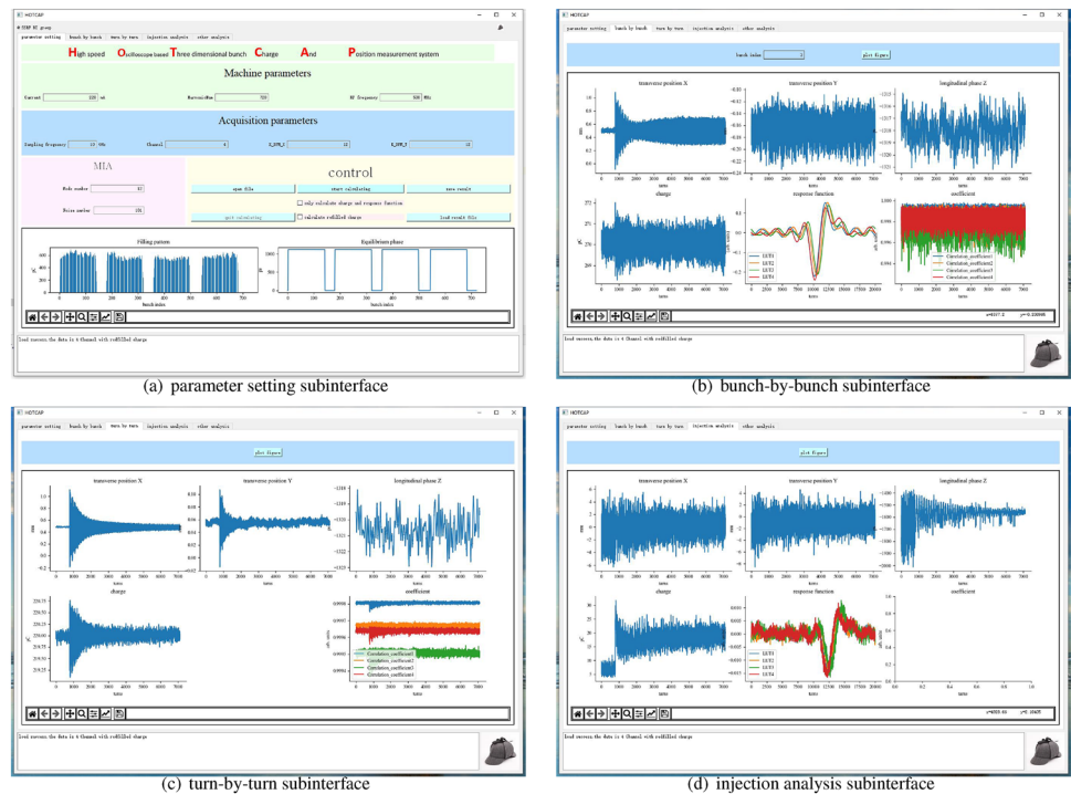
Fig. 6 (Color online) HOTCAP software package result display interfaces. The example data were recorded on July 25, 2020, at the SSRF: a parameter setting subinterface; b bunch-by-bunch subinterface; c turn-by-turn subinterface; d injection analysis subinterface
