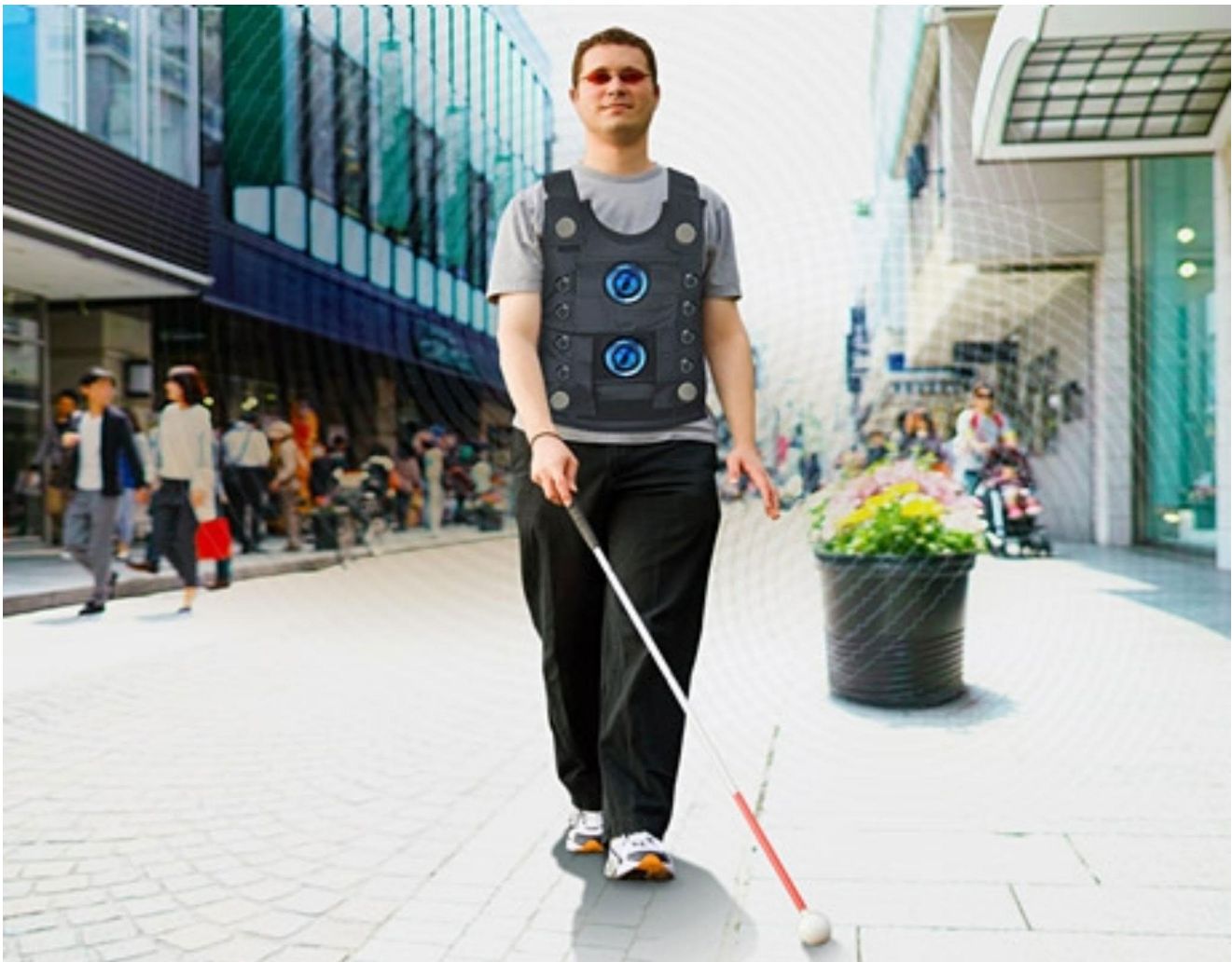
Fig. 9 Ultrasound sensors in different parts of the body to detect obstacles
