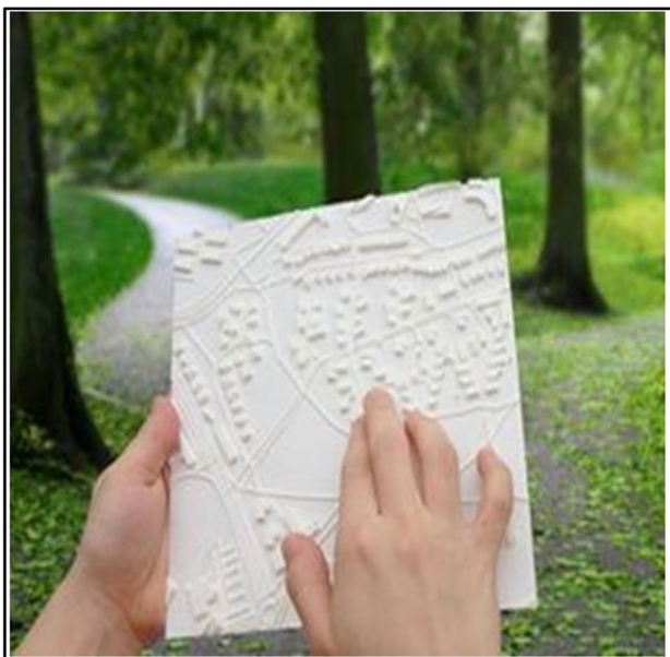
Fig. 4 3D tactile map made from OSM data
