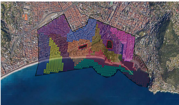
Fig. 10 Coverage example with the base methodology - in a non-convex polygon ROI - with NGZs - for 12 UAVs - with random initial positions
