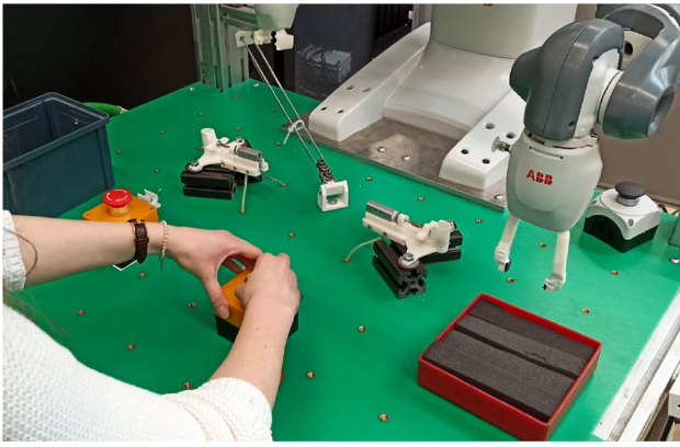
Fig. 8 An operator assembling the button in the shared workspace
