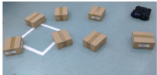
Fig. 9 The environment setup for this experiment. There are seven obstacles in a very small area ( 1.5 \text{ m} \times 1.5 \text{ m} ) and the goal of all the experiments is to let Turtlebot3 stop at the center of the white square which is 0.5 \text{ m} \times 0.5 \text{ m}
