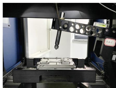
Fig. 1: Schematic diagram of MFT5000 friction and wear testing machine and pin-on-disc matching
