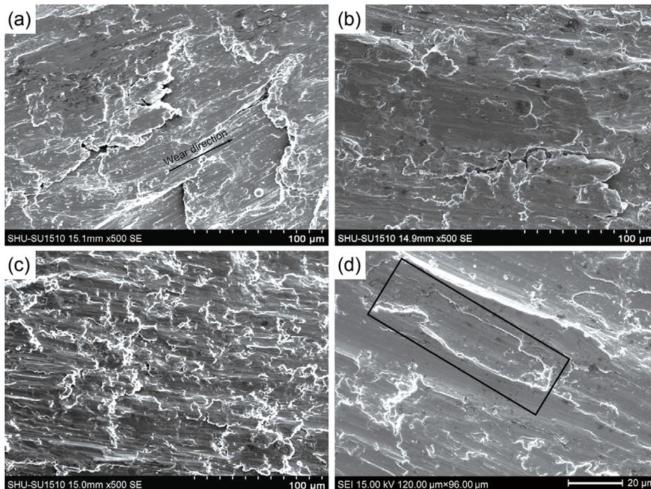
Fig. 3: Worn surface of normalized samples under condition of 30 N and 100 rpm for 30 min: (a) 0 Nb; (b) 0.2% Nb; (c, d) 0.4% Nb
