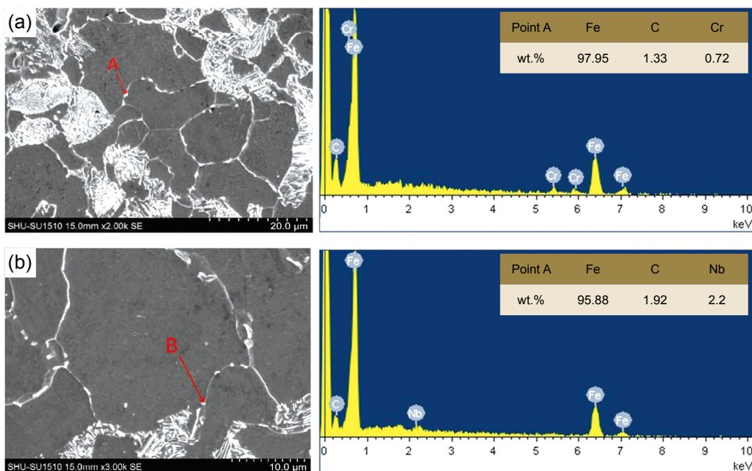
Fig. 5: SEM morphology and energy spectrum of normalized steel samples with different Nb contents: (a) 0 Nb; (b) 0.2% Nb
