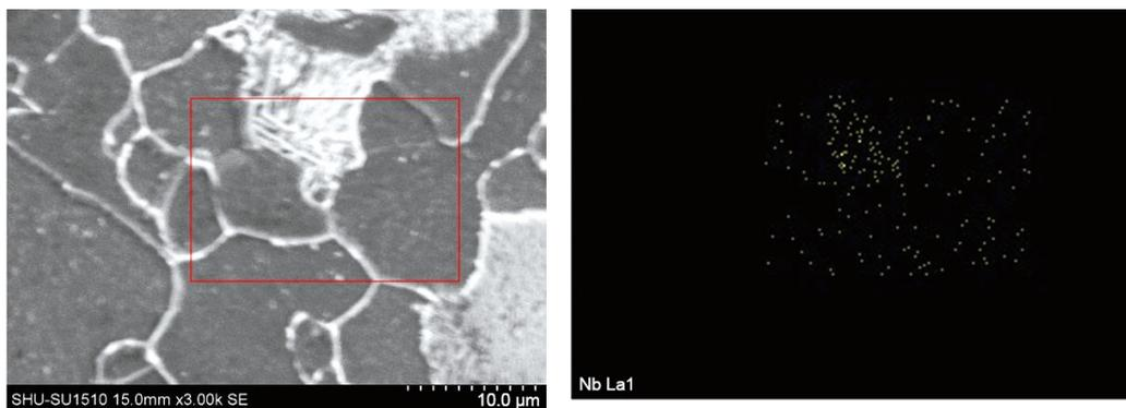
Fig. 9: Scanning energy spectrum of niobium element on the surface of 0.4% Nb normalized sample
