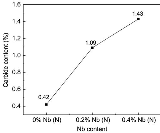
Fig. 6: Carbide content in normalized steel samples with different Nb contents
