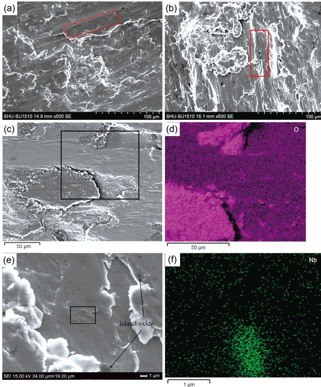
**Fig. 11: Wear morphology of 0.2% Nb normalized samples: (a) 50 N-100 rpm; (b) 30 N-150 rpm; (c) 50 N-100 rpm-EDS; (d) EDS analysis of Nb in Fig. 11(c); rectangular frame (e); 30 N-150 rpm-EDS; (f) EDS analysis of Nb in Fig. 11(e) rectangular frame**
