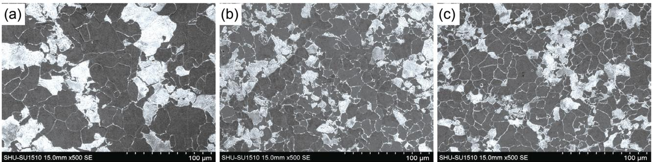
Fig. 4: SEM morphology of normalized samples with different Nb contents: (a) 0 Nb; (b) 0.2% Nb; (c) 0.4% Nb
