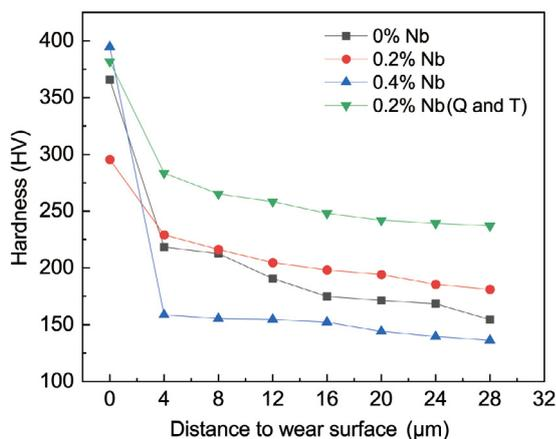
Fig. 10: Microhardness of specimen section with different Nb content
