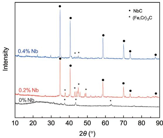
Fig. 7: XRD analysis of carbides in different Nb content normalized steels
