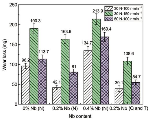
Fig. 2: Wear loss of experimental steels with different Nb contents
