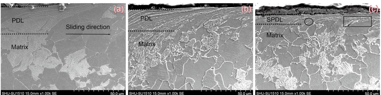
Fig. 8: SEM analysis of wear section: (a) 0 Nb; (b) 0.2% Nb; (c) 0.4% Nb
