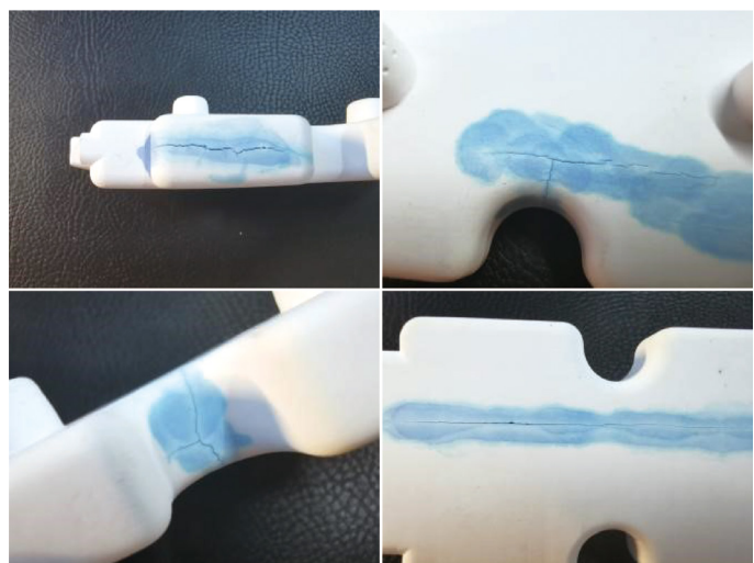
Fig. 11: Cracks of the solid core sample occurring during sintering
