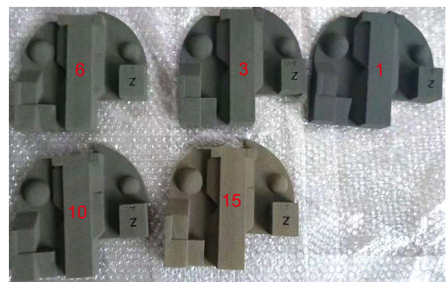
Fig. 4: Image of 3DP sand specimens with different gel times
