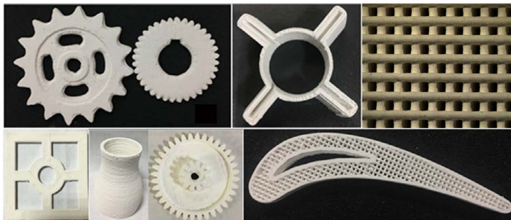
Fig. 20: Some typical ceramic samples prepared by LEF method
