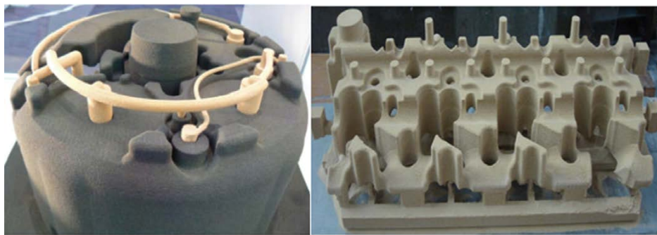
Fig. 1: Typical sand mold (core) prepared by 3DP method
