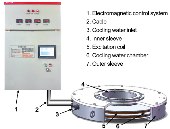
Fig. 1: Schematic diagram of magnetic field generation system
