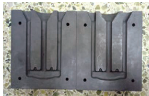
Fig. 1: Profile and geometry of high strength graphite mold
