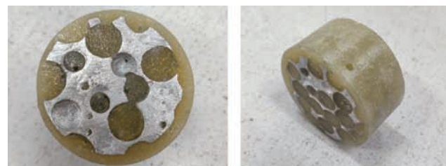
Fig. 2: Specimens of spherical open-cell aluminum foam-polyurethane composite
