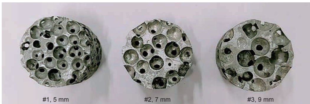
Fig. 1: Aluminum foam specimens with different pore sizes
