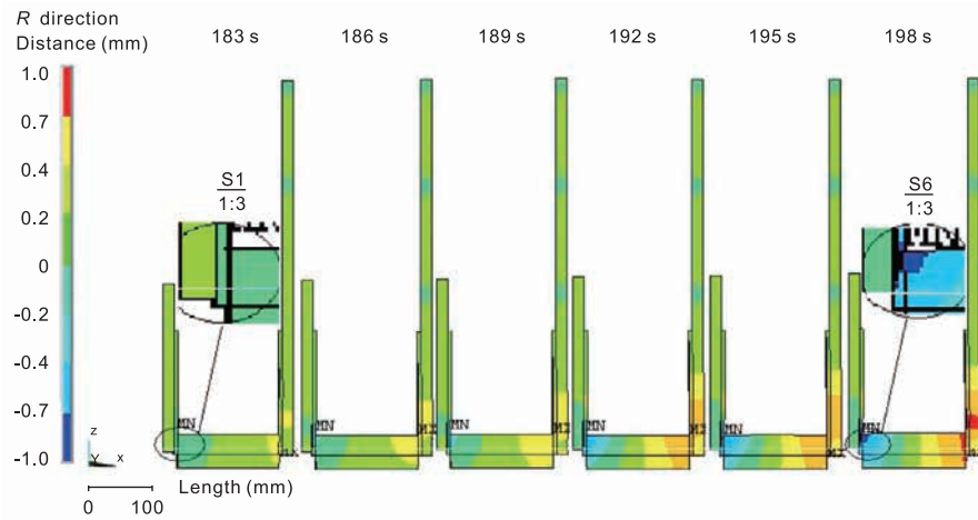
Fig. 11: EUPIM radial deformation at 180–198 s after up-pulling
