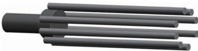
Fig. 2: Model of consumable electrodes for ESC hollow casting
