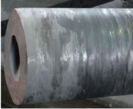
Fig. 14: \Phi 550/\Phi 220 ESC hollow cylindrical casting manufactured by EUPIM
