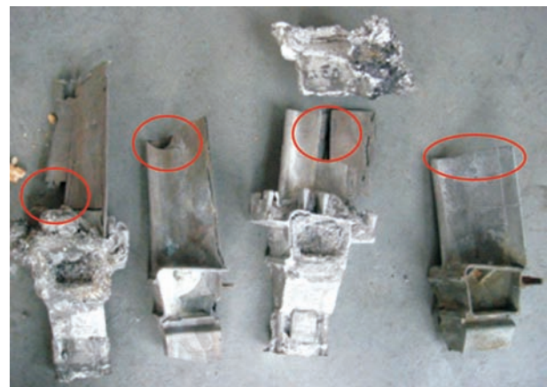
Fig. 4: Broken hollow turbine blades (made by high strength ceramic shell)
