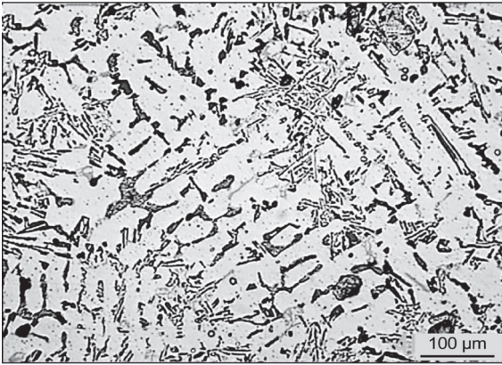
Fig. 3: Microstructure of AlSi9Cu1 (0.27% Fe) alloy modified with Sr
