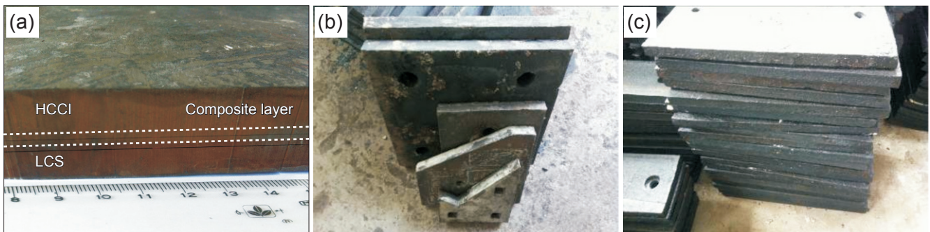
Fig. 7: Liquid-liquid bimetal LCS/HCCI composite wear plate: (a) wear plate macrostructure; (b) different shapes of wear plate; (c) deformed wear plate
