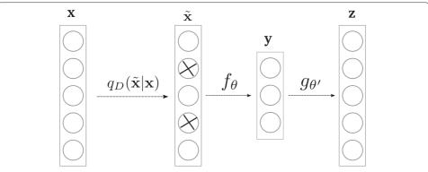
**Fig. 2** Denoising Autoencoder. A corrupted instance  $\tilde{x}$  of a graph  $\mathbf{x}$  is fitted into the Autoencoder's input. The Autoencoder is trained to recover a cleaned version of the input by compressing it through a non-linear mapping  $f_{\theta}$  and mapping it back (through  $g_{\theta'}$ ) to a reconstructed version of the original input graph  $\mathbf{x}$
