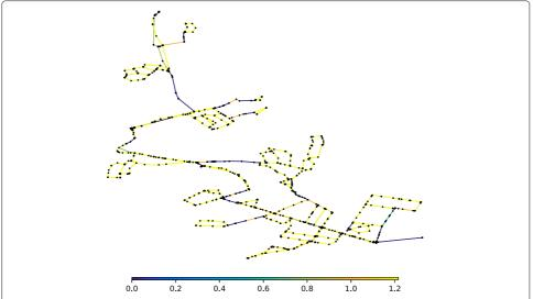
**Fig. 9** Reserve capacity of BWFL core links. Only the reserve capacity of BWFL core links is computed. The hydraulic model based analysis still requires to be run on the full model, to account for head losses in the forest links. The darker the link, the more critical
