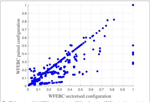
**Fig. 13** Comparison of link WFEBC values in the paired DMA configuration of BWFL against the sectorised configuration. The average decrease in FEBC indicates an improvement with regards to resilience in the paired configuration compared to the sectorised topology
