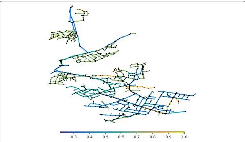
**Fig. 5** Analysis of the roughness of BWFL pipes. The colour of the links represent the normalised roughness coefficient of the pipes. Compared to Net3, BWFL is geographically heterogenous with regards to pipe roughness
