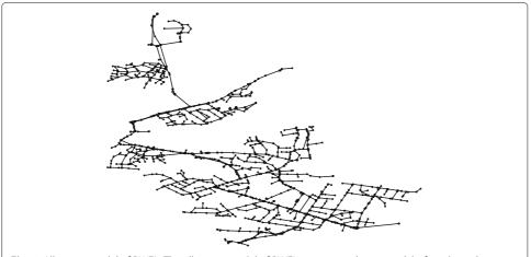
**Fig. 6** All mains model of BWFL. The all mains model of BWFL represents the network before the reduction step is undertaken
