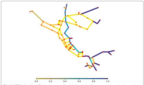
**Fig. 2** WFEBC of Net3 links. The betweenness of each link is weighted by customer demand and normalised by the maximum total flow it would have to support if there were no alternative paths to yield a measure of WFEBC. The darker the link, the more critical
