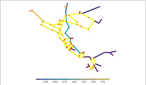
**Fig. 3** Reserve capacity of Net3 links. A hydraulic CLA is carried out to measure the reserve capacity of Net3 associated with the individual failure of each link. Reserve capacity measures the fraction of the total demand the network can supply while meeting pressure requirements. The darker the link, the more critical
