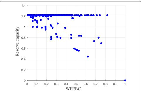
**Fig. 10** Analysis of the correlation between reserve capacity and WFEBC links values for BWFL. The reserve capacity of the individual links of the core model of BWFL is plotted against their WFEBC value
