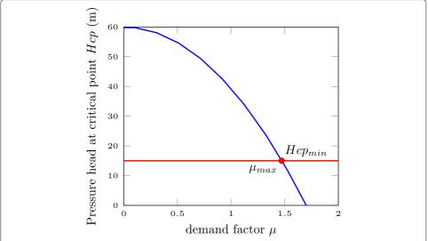
**Fig. 1** Definition of reserve capacity. As the demand factor  $\mu$  increases, the pressure head at the critical node decreases, until it reaches the minimum allowed pressure. The value of  $\mu$  when the pressure head at the critical point reaches the service head defines the reserve capacity of a network
