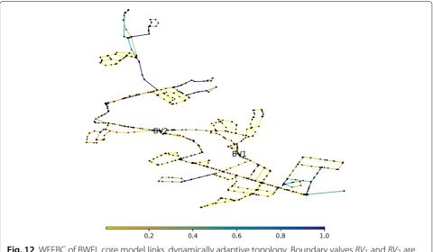
**Fig. 12** WFEBC of BWFL core model links, dynamically adaptive topology. Boundary valves  $BV_1$  and  $BV_2$  are opened to assess the resilience of the paired DMAs
