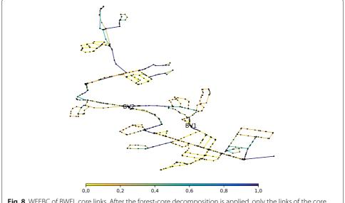
**Fig. 8** WFEBC of BWFL core links. After the forest-core decomposition is applied, only the links of the core model of BWFL are analysed. The darker the link, the more critical
