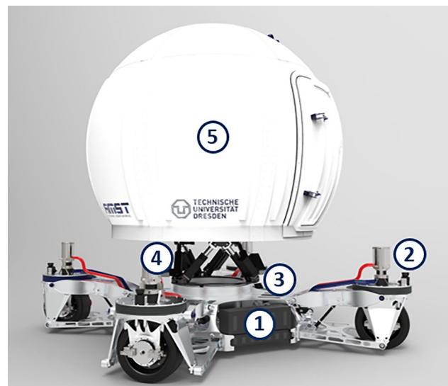
Fig. 1 Concept of the self-propelled driving simulator ©AMST-Systemtechnik GmbH
