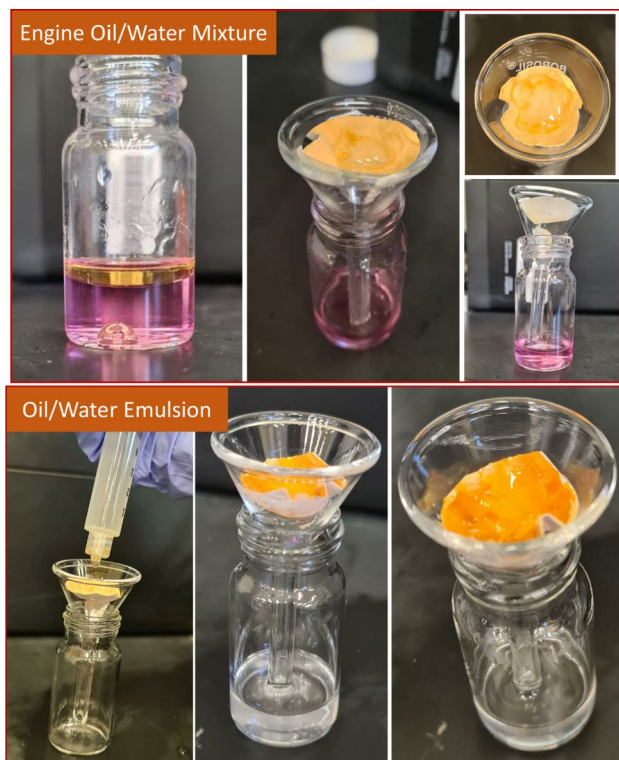
Fig. 7 Separation process for the oil/water mixture and the oil/water surfactant stabilized emulsion by the PSf-FeO/HNT nanocomposite modified PES support membrane by gravity driven separation process
