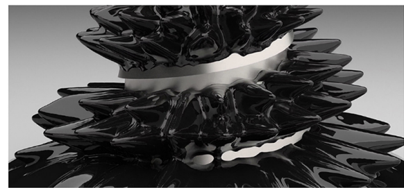
Fig. 48 A ferrofluid climb up a steel helix under a strong external upward magnetic field to create surface spikes. Reproduced with permission from Ref. [305], © Owner/Author 2019.
