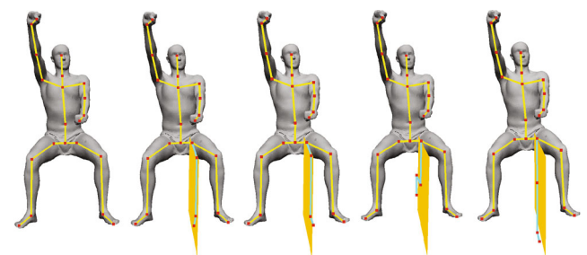
Fig. 4 Steps in rotating leg and foot bones to the standard pose. Reproduced with permission from Ref. [35], © Springer Science+Business Media, LLC, part of Springer Nature 2020.
