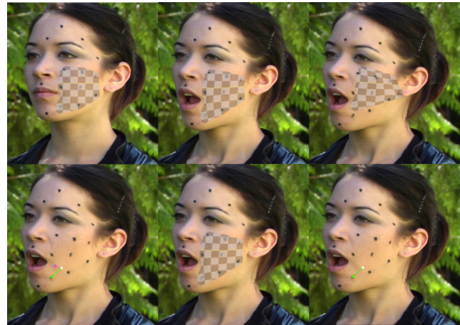
Fig. 6 Correcting tracking errors caused by large displacements. Top left to bottom right: part of reference frame 1 with tracking region marked, frame 12 with tracking from reference still working, frame 13 with tracking directly from frame 1 failing, provision of a single correspondence as hint (green), correct tracking with additional hint, and estimated displacement vector for corrected point.
