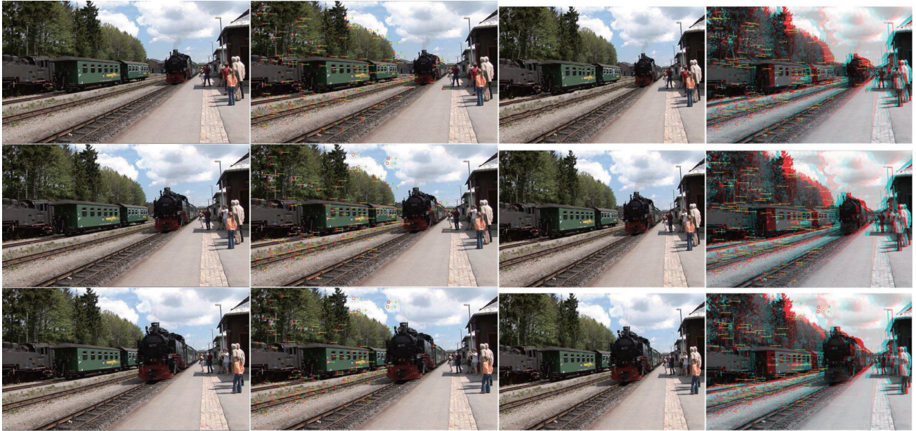
Fig. 3 Resolution adaptation and depth remapping for the frame sequence. Left to right: original left frames ( 720 \times 416 ), original disparity at the key points, left frames at target resolution ( 600 \times 400 ), increased disparity ( 1.5\times ).
