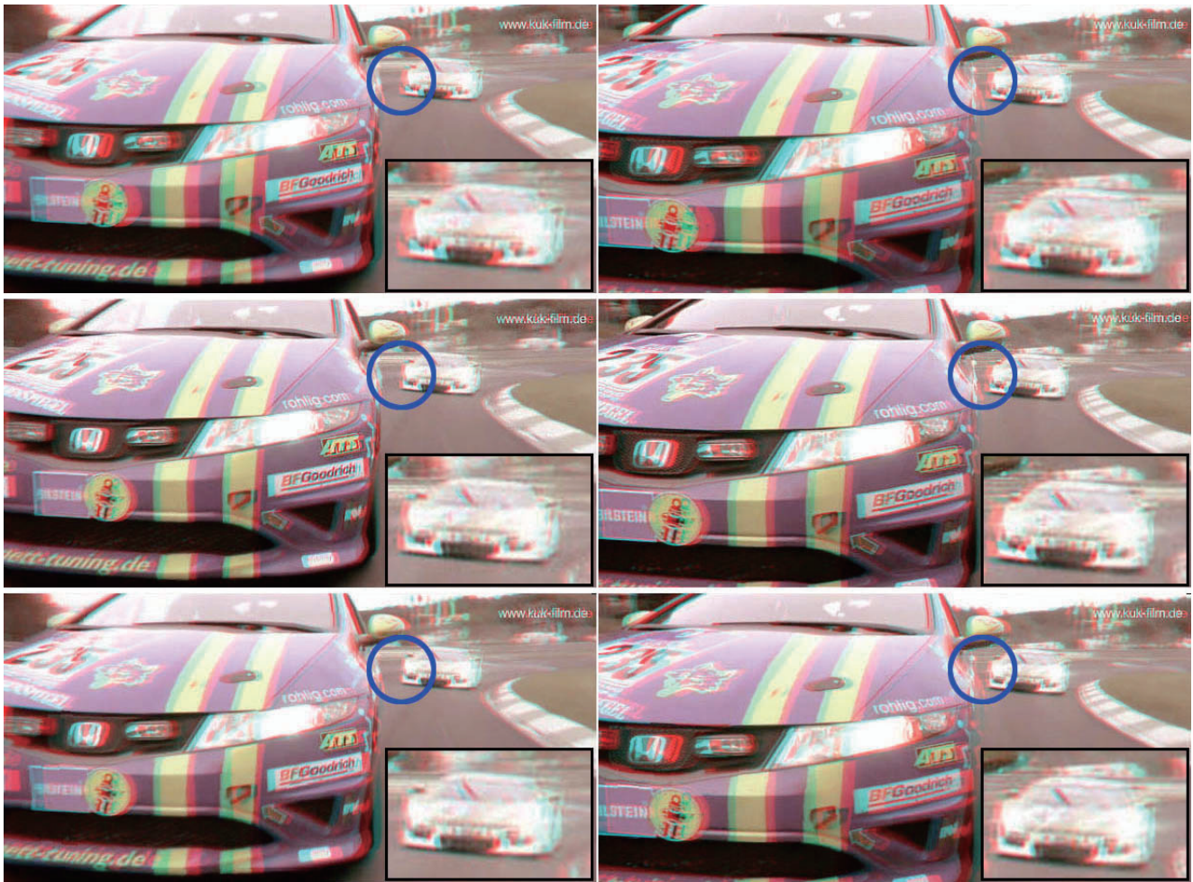
Fig. 6 Comparison of retargeting results. Top two images: two sequential original frames. Middle two images: results computed by the method in Ref. [21]. Bottom two images: results computed by our method. The objective is to reduce the disparity to lie within the comfort zone. In the blue circle, the disparity changes obviously when using Ref. [21]. Using our method, the disparity variation is more consistent with the original video.
