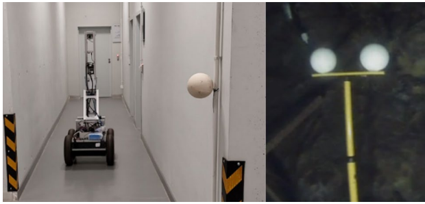
Fig. 17 References object on robot path in the building corridor (left) and in the underground tunnel area (right)
