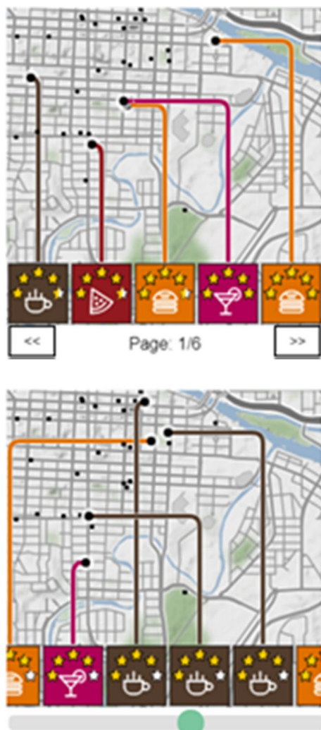
Fig. 22 Two labeling models allow a user to access labels for all points on a map without zooming into a very large scale. Top: A model allowing a user to navigate from page to page. Bottom: A model based on a slider that can be used to let labels enter or leave the map (Image taken from a mobile application, leading to a reduced resolution)
