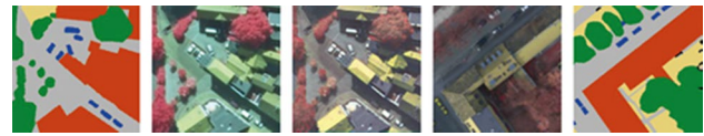
Fig. 6 Result of deep domain adaptation using the method of (Wittich and Rottensteiner 2021). From left to right: Classification of source domain image, source domain image, source images transformed to the target domain by the AAN, target domain image, classification of target domain image
